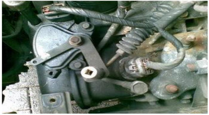
ONCE THESE NUTS ARE UNDONE THE CABLE WILL BE STUCK WITH GLUE (CENTRE)
